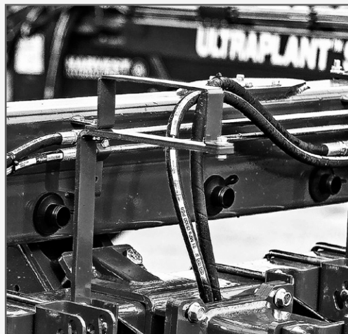
INTR-AIRWAY vac port located inside 9x5 tube Keeps bar free of extra lines, cleaner for maintenance & service
