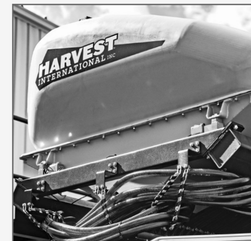
CSD Scale Option; weighs each tank 8 load cells to weigh each tank independently. In-cab readout.
