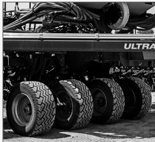
FR model SuperMuck Center Tires [445/50R22.5] Available with 40' & 60' front running bars only.
